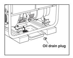
Use fresh and high quality lubricating oil to the specified level as directed on page 7. If contaminated or deteriorated oil is used or the quantity of the engine oil is not sufficient, the engine damage will result and its life will be greatly shortened.
